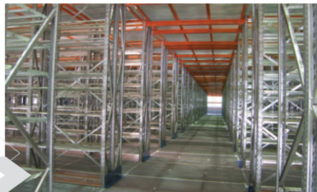
Multi-storey structure designed on the basis of X-S Max shelf racks.
